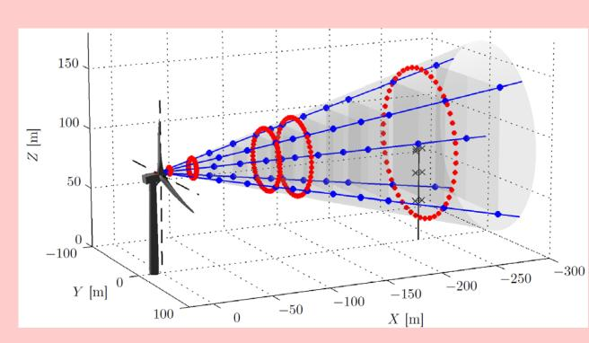
Fig.3. Scanning pattern for each lidar at Nørrekær Enge (Avent 5 beam : blue; ZephIR DM: red)
