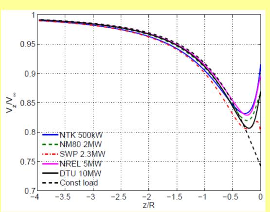
Fig.1. Simluated wind velocity as function of distance upstream of the rotor for 5 different turbines
