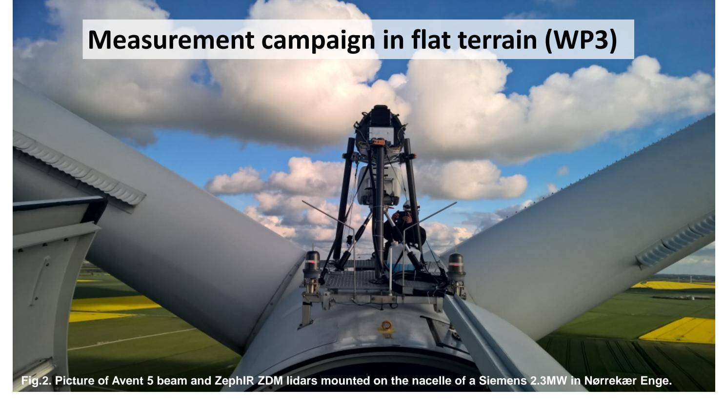
Both calibrated nacelle lidars have been installed on a Siemens 2.3MW wind turbine in the Nørrekær Enge wind farm, surrounded by flat terrain, in Denmark. A met mast, compliant to the IEC 61400-12-1:2005 requirements, has been used as reference wind speed measurement. Moreover the turbine has been instrumented for a full load assessment including strain gauges on the blade roots and the top and bottom of the tower.
