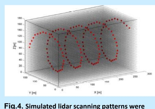
Fig.4. Simulated lidar scanning patterns were implemented by imposing constraints on randomly generated Gaussian turbulence fields.)
