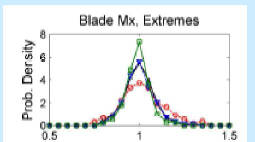
Fig.5. Probability density of uncertainty in blade root out of plane extreme loads. (Red: unconstrained; Blue: constrained with ZephIR DM pattern; Black: cinstrained with Avent 5 Beam pattern)
