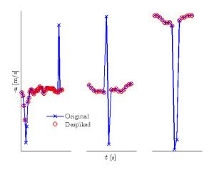
Fig. 3 Examples of successfully removed spikes.
