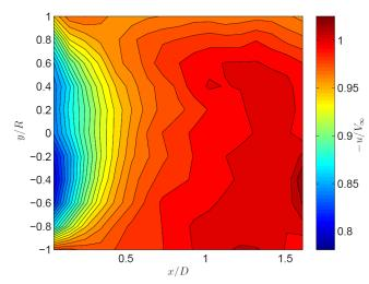
Fig. 5 Contours for  $-u/V_{\infty}$  for inlet velocities 9.6 <  $u_{\infty}$  < 10.2 m/s
