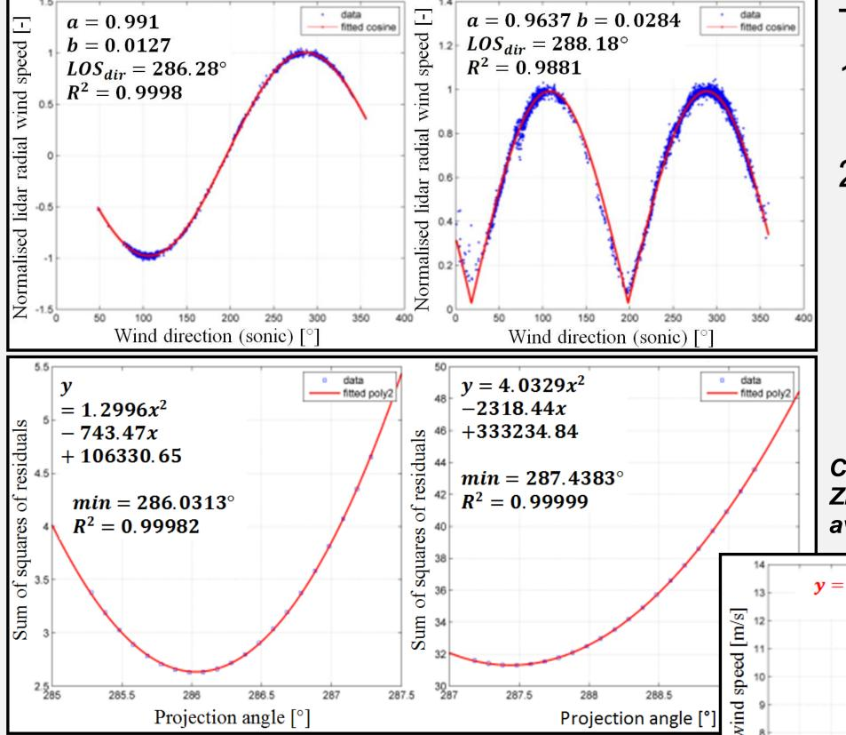
The LOS direction is estimated by: 1. Fitting the lidar response to the wind direction.
