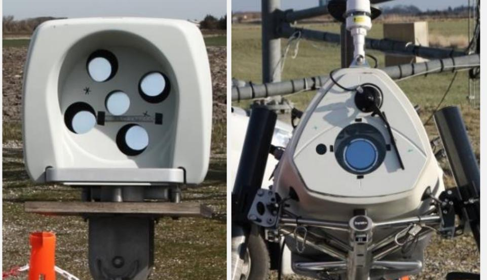
fundamental reason for The calibration developing procedures is assign to uncertainties to lidars wind Commercial measurements. applications of lidars, e.g. power performance testing or resource demand the assessment, estimation of measurement uncertainties.
