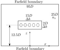
**Figure 3.** Frontal view of the numerical domain.
