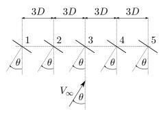
Figure 1. Schematic of the wind turbines' arrangement and reaction to changing inflow directions.
