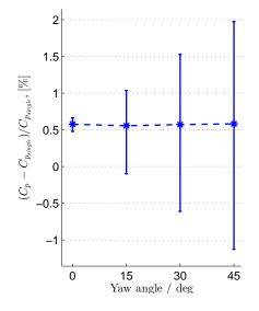
Figure 5. Percentage change in the power coefficient for different yaw angles.
