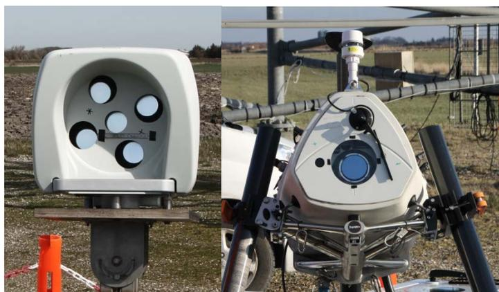
**Figure 1. Wind profiling lidar examples: 5-beam AventLidar Demonstrator (left) and Zephyr DM (right)**
