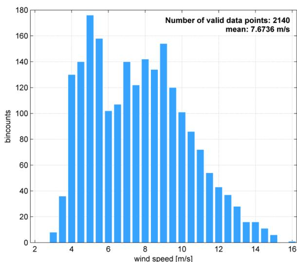
Figure 17. Distributions of radial wind speeds after filtering
