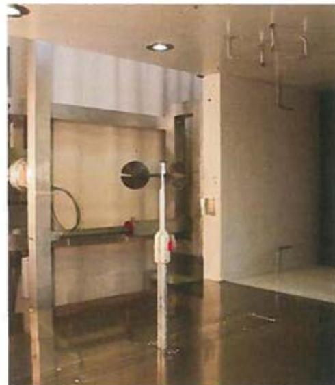
Calibration set-up of the anemometer calibration in the wind tunnel of Deutsche WindGuard, Varel. The anemometer and orientation shown may differ from the calibrated one. Remark: The proportion of the set-up is not true to scale due to imaging geometry.
