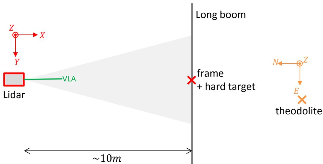
Figure 6. Top-view schematic of the measurement setup for geometry verification and tilt inclinometer calibration
