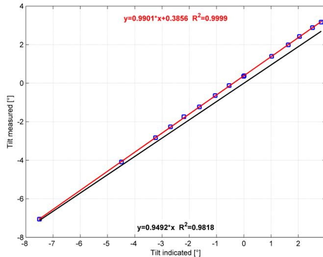
**Figure 12. Tilt calibration results: measured vs. lidar indicated**
