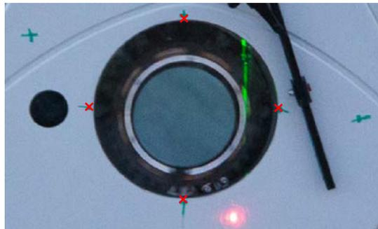
Figure 10. Measuring the geometry of ZDM lidar's window
