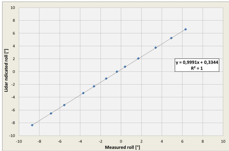
**Figure 9. Verification of the roll inclinometer gain**
