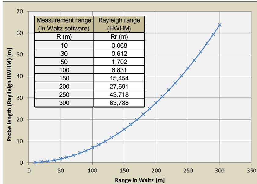
**Figure 4. Probe length model of ZDM lidar**
