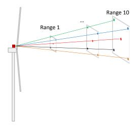
Figure 2. Schematic of the 5-beam lidar (Avent) mounted on the nacelle of a wind turbine
