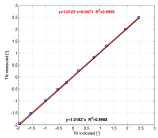
Figure 10. Tilt calibration results: measured vs. lidar indicated
