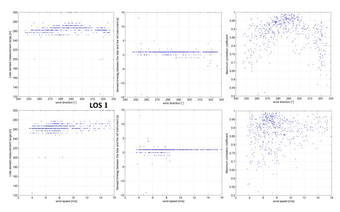
Figure 33. Sensed range and timelag verification for LOS 1
