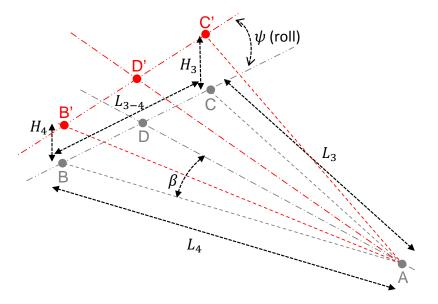
Figure 11. Schematic of the roll calibration measurement setup
