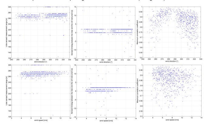
Figure 20. Sensed range and timelag verification for LOS 0. Left: sensed range [m]. Center: timelag [s]. Right: maximum correlation coefficient [-]. Top: vs. wind direction [°]. Bottom: vs. HWS [m.s<sup>-1</sup>]
