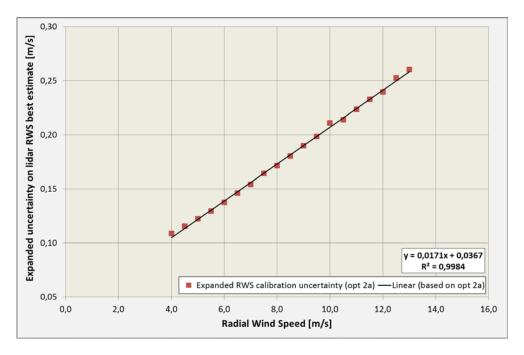
Figure 21. RWS calibration expanded uncertainty (LOS 0)
