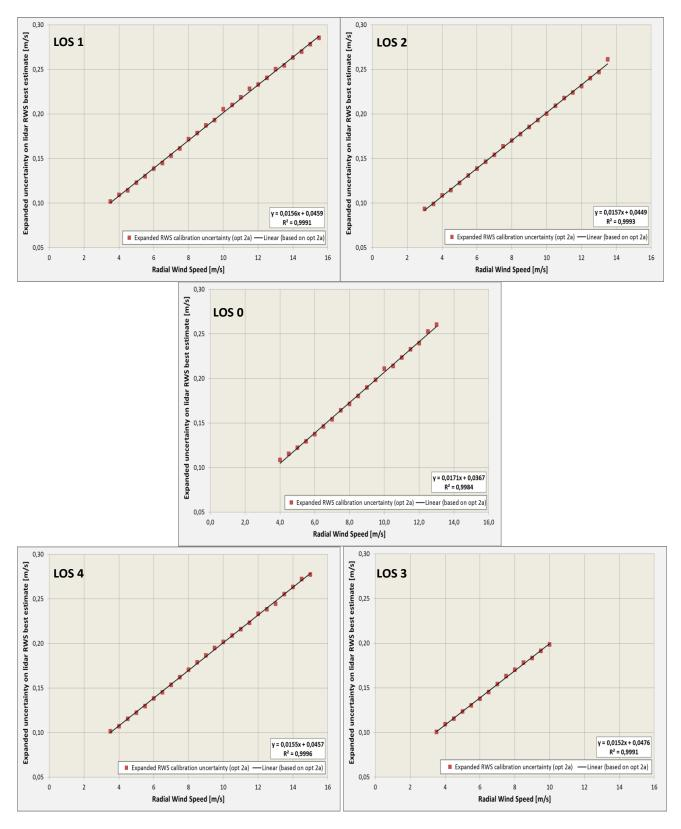
Figure 37. Expanded RWS uncertainty per bin – all 5 beams.
