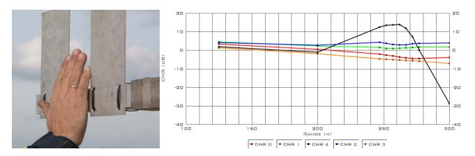
Figure 7. Shutters (left) and CNR response (right) of a pulsed lidar hitting a hard target at 255m: example of the 5-beam Demonstrator lidar (Avent).
