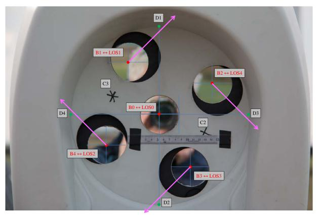
Figure 8. Geometry of the lidar's optical head windows
