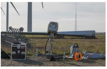
Figure 12. Roll calibration results: measured vs. lidar indicated (left). Photograph of the 5-beam Demonstrator lidar during the roll calibration, Høvsøre, DK (right).
