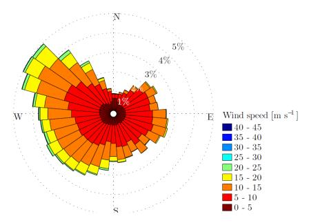
Figure 25. Wind rose at 100m in Høvsøre, between 2005-2013
