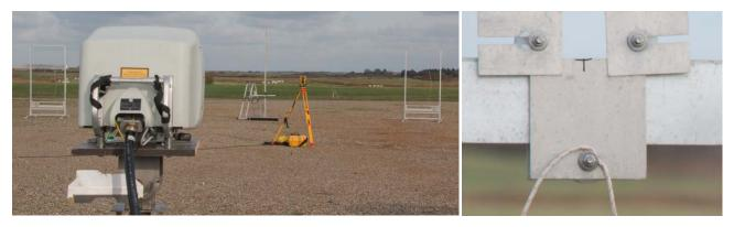
Figure 4. Left: photograph of the measurement setup for ground calibration of the 5-beam Demonstrator's inclimometers. Right: shutters for detecting the beam position by blocking/unblocking
