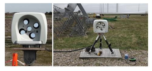
Figure 1. The 5-beam Demonstrator on a 3 axis-rotating platform (left) and its tripod (right), Høvsøre, DK
