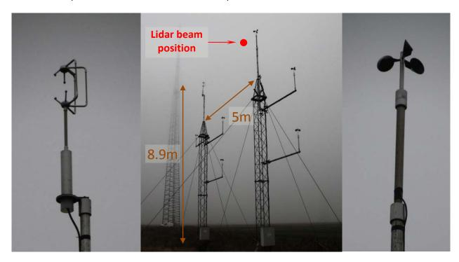
Figure 14. Reference instruments for RWS calibration: sonic anemometer (left), two masts (center), cup anemometer (right)
