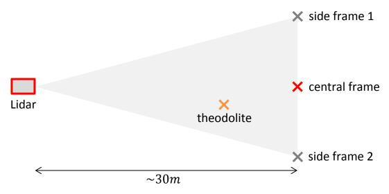
Figure 6. Top-view schematic of the measurement setup for inclinometers calibration
