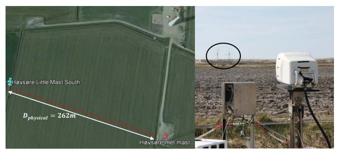
Figure 15. Calibration measurement setup of the Avent 5-beam Demonstrator lidar at DTU Wind Energy test site, Høvsøre (DK)
