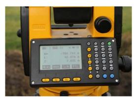
Figure 5. 3D coordinates measurements with a theodolite
