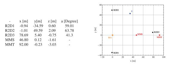
Figure 6: Coordinates (left) and the corresponding drawing (right) of the location of the 3 short-range WindScanner (R2D1, R2D2 and R2D3), the two met mast (MMS and MMT) and of the TST (T).
