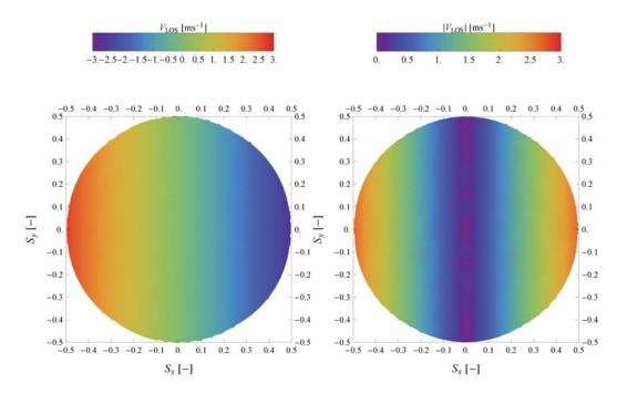
Figure 22: Simulated radial blade speeds as measured from a SpinnerLidar installed on the nacelle of a wind turbine, which is diplaced vertically along the z-axis (see Figure 19) from the center of rotation of the wind turbine's blades.
