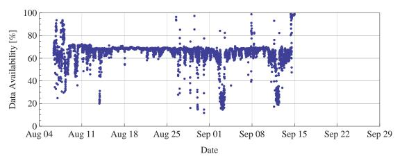
Figure 35: Data availability after filtering out speed measurements originated from the wind turbine's blades.
