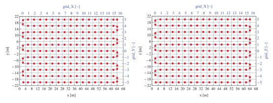
Figure 10: The horizontal plane scan #1 (left), the vertical plane scan #2 (right), the vertical plane parallel #3 (bottom) to the wind turbine rotor and their corresponding grids.
