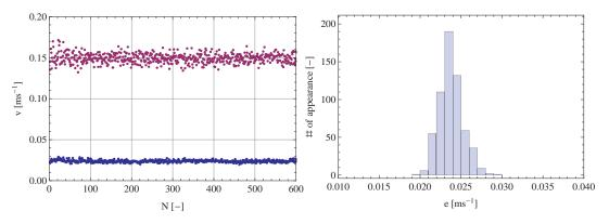
Figure 25: Estimated median value of the absolute error of the simulated radial blade speed in comparison to the measured ones (left) and the corresponding histogram (right).
