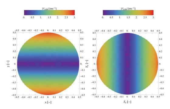
Figure 23: Simulated radial blade speeds as measured from a SpinnerLidar installed on the nacelle of a wind turbine, which is diplaced horizontally along the y-axis (see Figure 19) from the center of rotation of the wind turbine's blades..
