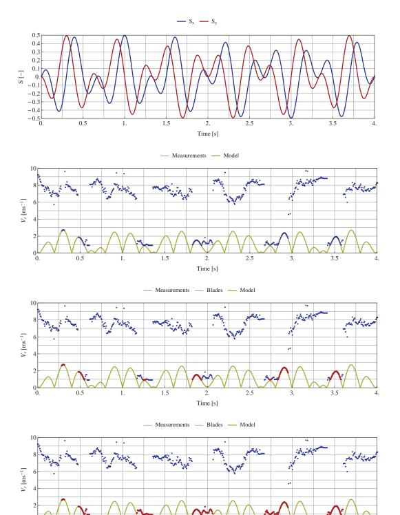
Time [s] Figure 27: Example of the implementation of the blade filtering algorithm.
