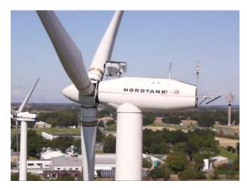
Figure 13: The SpinnerLidar installed on top of the NordTank turbine at DTU Risø campus.
