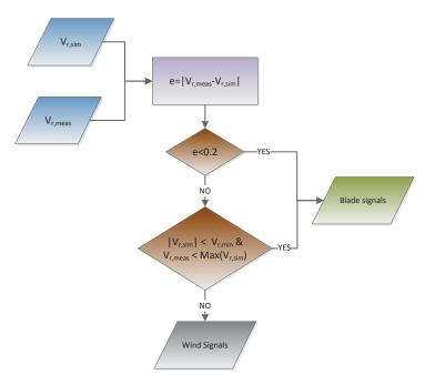
Figure 26: Architecture of blade filtering algorithm.
