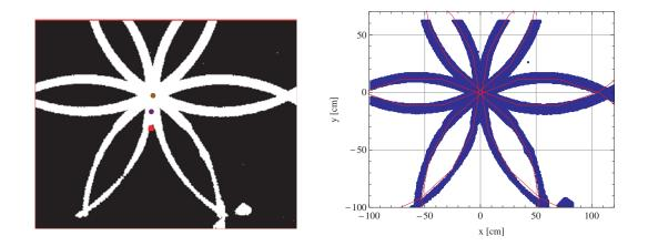
Figure 16: (Left) The scanning pattern of the spinnerLidar based on the trace of the laser beam which was monitered through the use of an IR camera. (Right) The measured scanning pattern (blue) in comparison with the theoretical expected scanning pattern (red).
