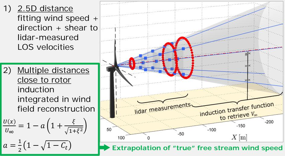
Lidar measurements @ multi-dist (near flow) Mast comparison, Nørrekær Enge campaign, 7 months
