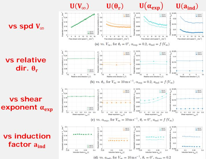
10 **DTU Wind Energy**, Figure 4.11: Profiling nacelle lidars MC results: expanded uncertainties  $U_{V_{\text{H}}}$ ,  $U_{\theta_{\text{r}}}$ ,  $U_{\alpha_{\text{exp}}}$ ,  $U_{a_{\text{ind}}}$  as a function of  $V_{\text{H}}$ ,  $\theta_{\text{r}}$ ,  $\alpha_{\text{exp}}$  and  $a_{\text{ind}}$ .
