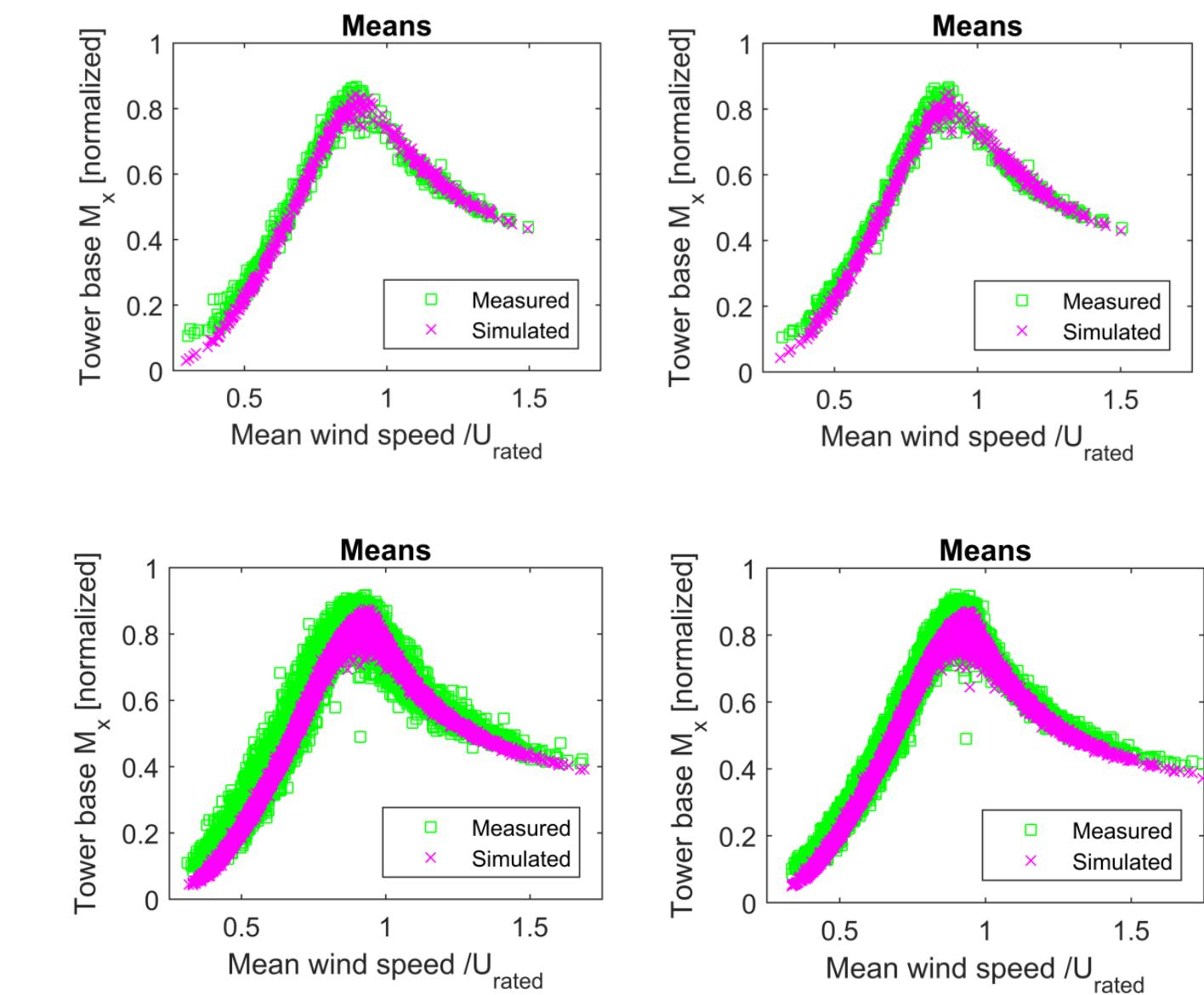
Figure 4. Comparison between measured and simulated mean tower base bending moment at Nørrekær Enge. Top left and right: comparison for narrow wind direction sector ( $102.9^\circ \pm 5^\circ$ ). Bottom left and right: comparison for wide wind direction sector ( $96^\circ - 225^\circ$ ). Left: using statistics from mast data, right: using lidar-derived statistics.
