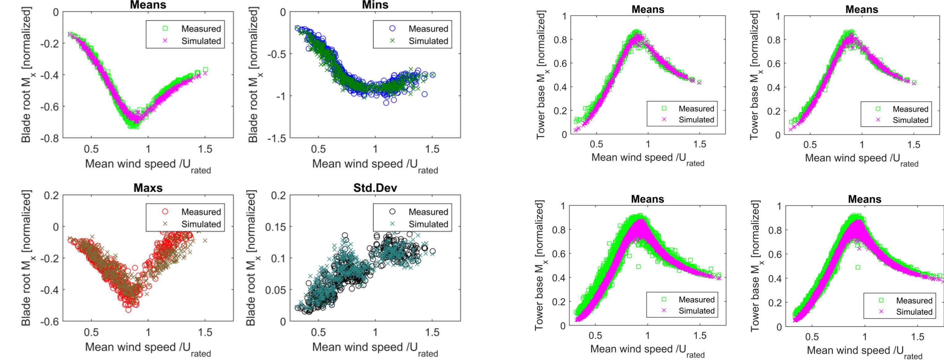
Figure 3. Comparison between measured and simulated blade root flapwise load statistics for a narrow wind direction sector ( $102.9^\circ \pm 5^\circ$ ) at Nørrekær Enge. Simulation inputs are derived using a 5-beam nacelle-mounted lidar.
