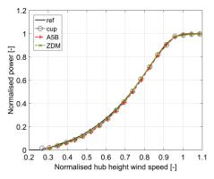
Figure 3: Measured power curves (binned data).
