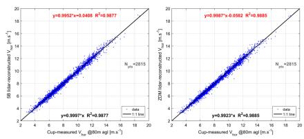
Figure 1: Comparison between mast-measured and lidar-estimated horizontal wind speed at hub height and 2.5D upstream using short-range measurements. Left: 5B-Demo lidar. Right: ZDM lidar.
