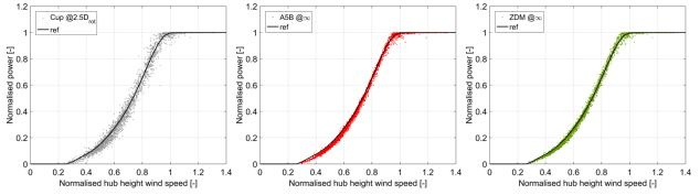
**Figure 2**: Measured power curves (10-min data). Left: mast-mounted cup. Middle: 5B-Demo lidar, using  $V_{\infty}$  estimates. Right: ZDM lidar, using  $V_{\infty}$  estimates.
