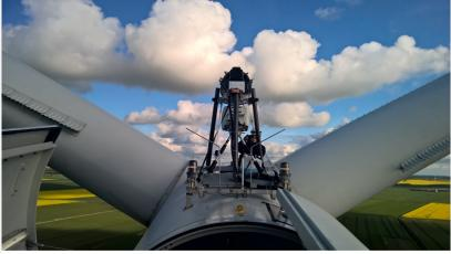
Lidars view from the nacelle of turbine 04, Nørrekær Enge, DK (MC2, WP3) 7 DTU Wind Energy, Technical University of Denmark
