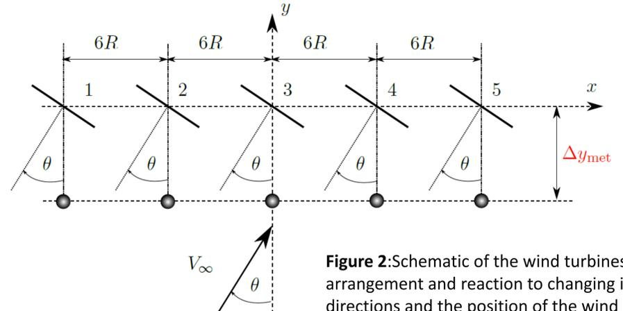
**Figure 2:** Schematic of the wind turbines' arrangement and reaction to changing inflow directions and the position of the wind speed measurements
