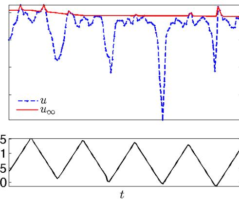
Fig. 2 Example of streamwise velocity component time series ( $u$ ) and inlet velocity ( $u_{\infty}$ ) for a single scan.  $D$  represents the diameter of the turbine.
