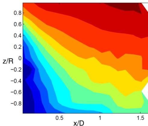
Fig. 6 Contours of  $-u$  for  $10.0 < V_{met} < 12.0$  m/s and  $0^\circ < \theta < 5^\circ$ .
