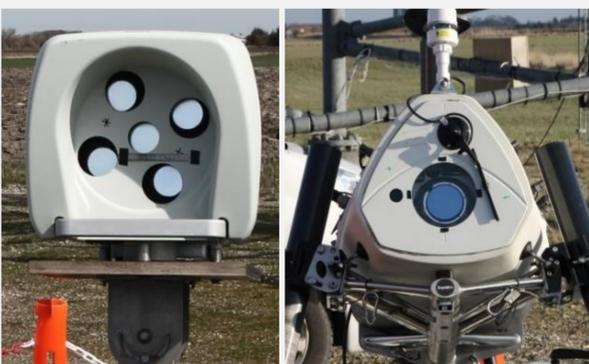
Pictures of the 5-beam Demonstrator (left) and the Zephyr Dual Mode (right), during their calibration at DTU Wind Energy test site, Høvsøre, DK
