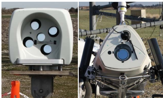
Fig. 1 Left: 5-beam Demonstrator (Avent Lidar Technology), right: ZephIR Dual Mode (ZephIR lidar)
