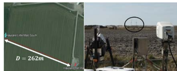
Fig. 2 Calibration measurement setup of ZDM (left) and the 5-beam Demonstrator (right), DTU Wind Energy test site, Høvsøre (DK)
