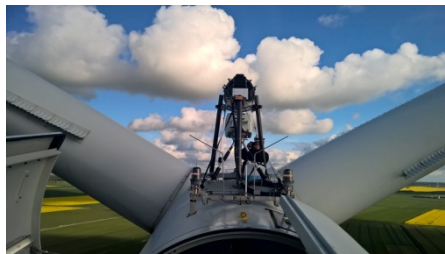
Lidars view from the nacelle of turbine 04, Nørrekær Enge, DK (MC2, WP3)
