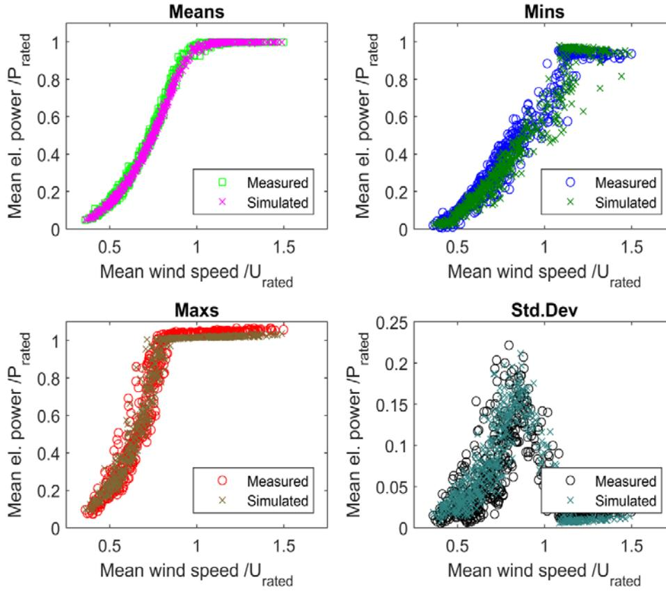
Good reproduction of power production and its variability as well as fatigue damage equivalent loads
