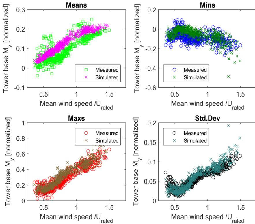
Simulated tower base side-side and blade root edge loads match measurements much better.
