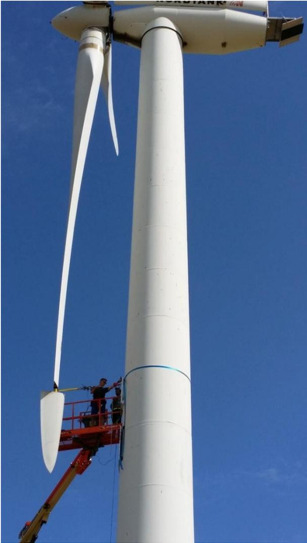
**Figure 15** Picture of one of the blade being attached to the tower for the flapwise bending moment strain gauge calibration
