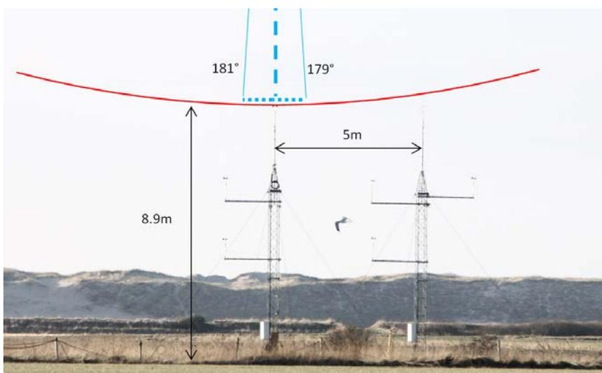
**Figure 13. Averaging LOS velocity measurements in a narrow azimuth sector (ZDM lidar)**
