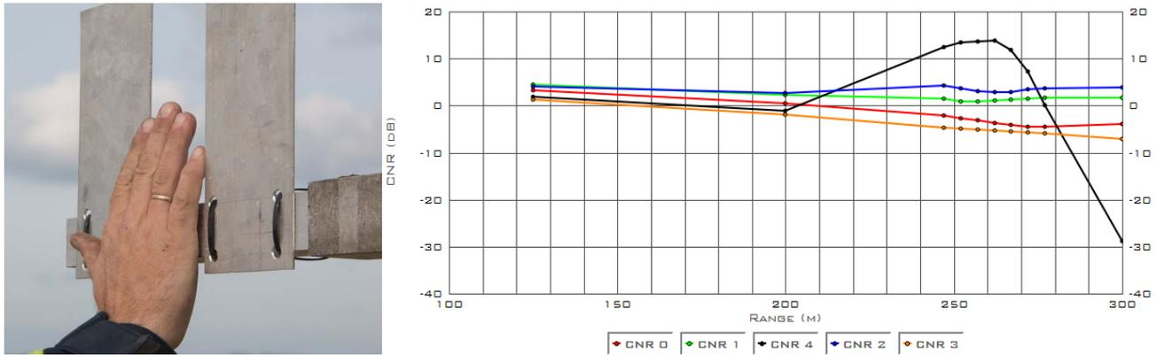
Figure 3. Shutters (left) and CNR response (right) of a pulsed lidar hitting a hard target: example of the 5-beam Demonstrator (Avent).
