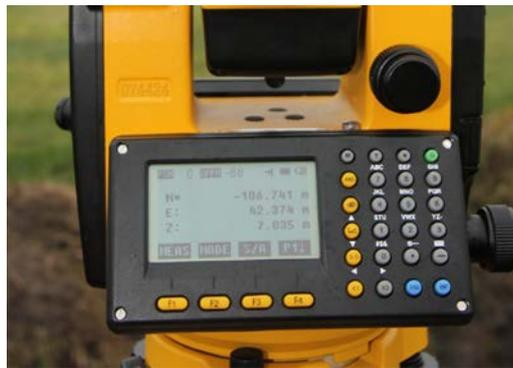
Figure 5. 3D coordinates measurements with a theodolite
