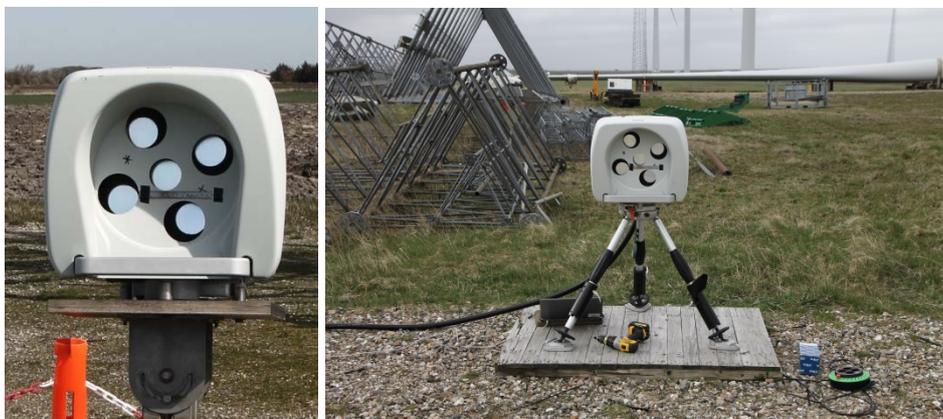
**Figure 1. The 5-beam Demonstrator on a 3 axis-rotating platform (left) and its tripod (right), Høvsøre, DK**
