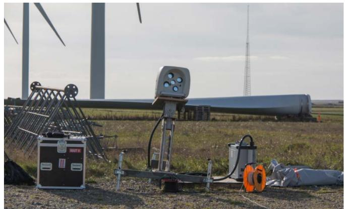
**Figure 12. Roll calibration results: measured vs. lidar indicated (left). Photograph of the 5-beam Demonstrator lidar during the roll calibration, Høvsøre, DK (right).**
