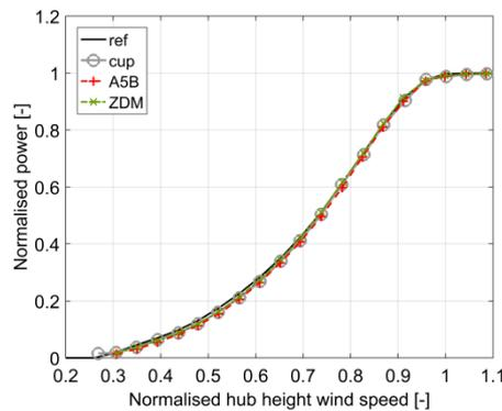
**Figure 3:** Measured power curves (binned data).
