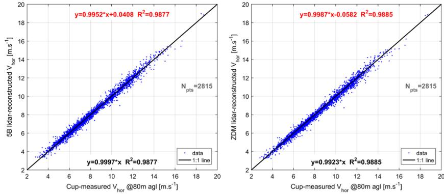
**Figure 1:** Comparison between mast-measured and lidar-estimated horizontal wind speed at hub height and 2.5D upstream using short-range measurements. **Left:** 5B-Demo lidar. **Right:** ZDM lidar.
