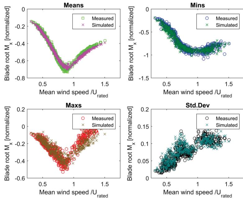
**Figure 3.** Comparison between measured and simulated blade root flapwise load statistics for a narrow wind direction sector ( $102.9^\circ \pm 5^\circ$ ) at Nørrekær Enge. Simulation inputs are derived using a 5-beam nacelle-mounted lidar.
