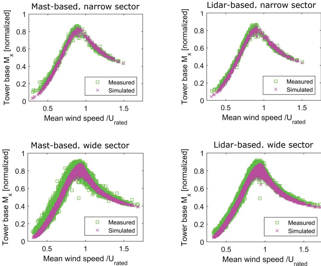
**Figure 4.** Comparison between measured and simulated mean tower base bending moment at Nørrekær Enge. Top left and right: comparison for narrow wind direction sector ( $102.9^\circ \pm 5^\circ$ ) for mast-derived and lidar-derived statistics respectively. Bottom left and right: comparison for wide wind direction sector ( $96^\circ - 225^\circ$ ). Left: using statistics from mast data, right: using lidar-derived statistics.
