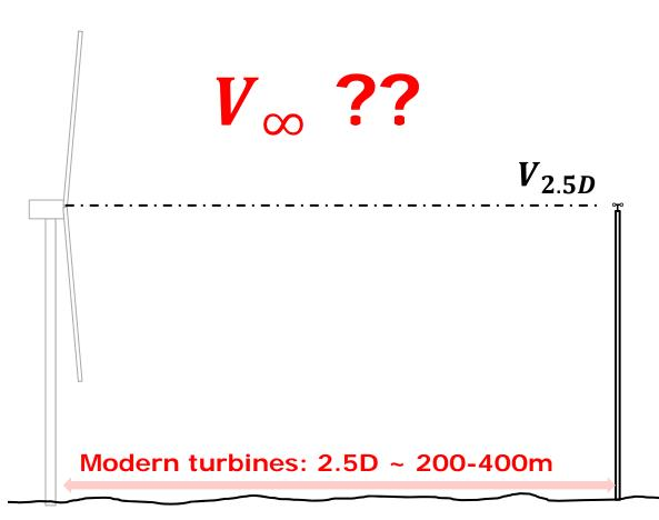
Turbine testing requires to relate power and loads to "free wind speed".
