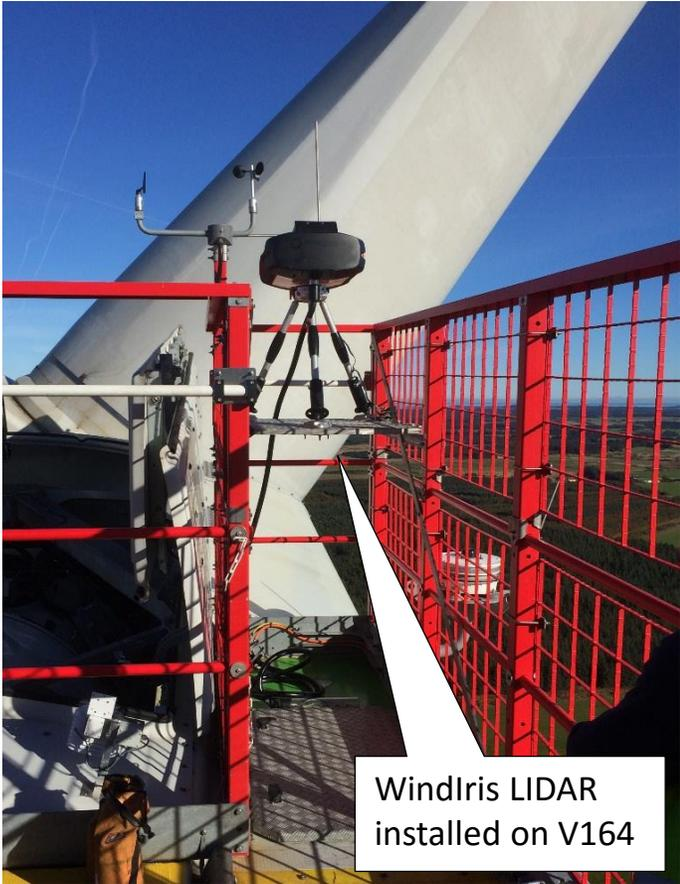
WindIris LIDAR installed on V164
