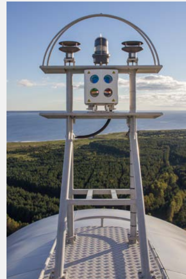
Wind Eye (4-beam) by Windar Photonics
