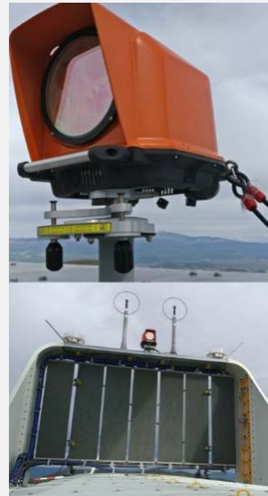
Wind Iris (4-beam) by AventLidar
