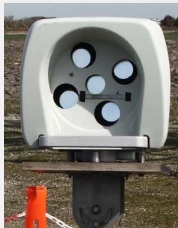
Avent 5-beam Demonstrator (5B-Demo): pulsed, step-staring
